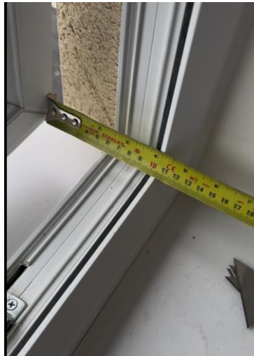
Figure 5: Measurement of window position, illustrating 100 mm stroke length
